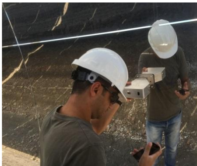
Picture: Measurement of soiling and cleanliness at parabolic trough solar mirror with pFlex mobile device
