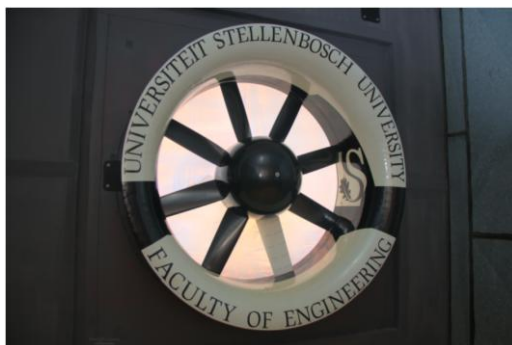
Figure 2: Small-scale fan in BS848 fan test facility (Louw, 2015)
