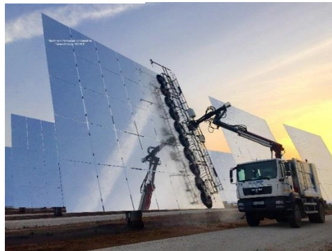
Pictures 3-5: Innovative brush system developed by ECILIMP guarantees full cleaning coverage of the mirror surface
