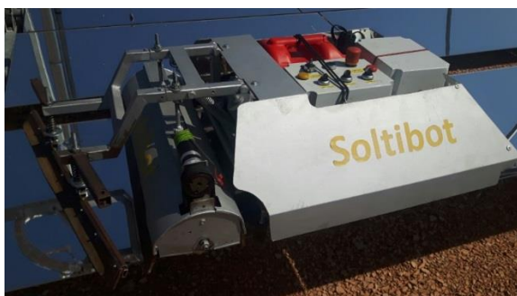
Picture 8: Prototype robot called “Soltibot” developed by SOLTIGUA for cleaning of Linear Fresnel (© Soltigua)
