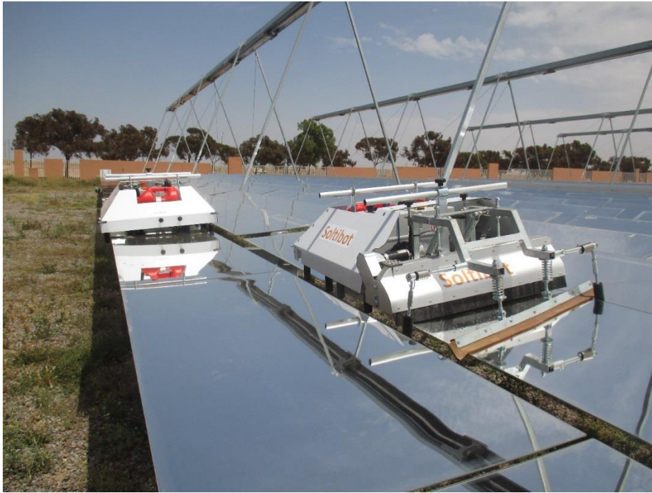
Picture: Cleaning robot "Soltibot"® developed by Soltigua tested on Linear Fresnel at Green Energy Park in Morocco (Copyright: Soltigua)
