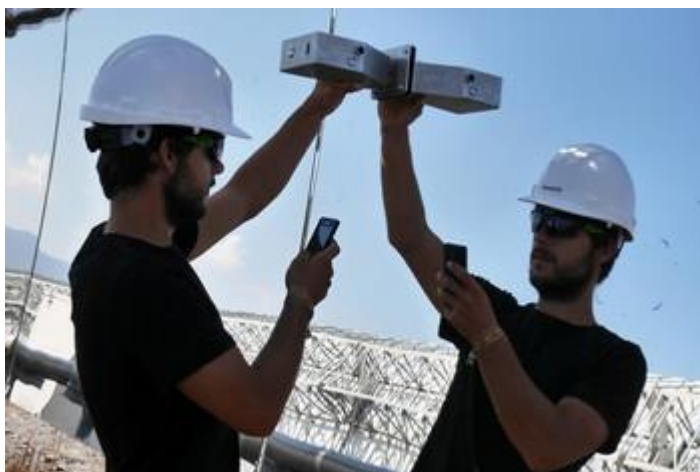
Measuring soiling in the solar power plant with the mobile reflectometer pFlex. © Fraunhofer ISE.
