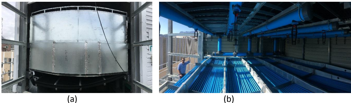
Figure 6: A (a) frontal view and (b) view from in between the bundle and sprayers of the deluge test section (© ENEXIO Management GmbH, Kelvion Thermal Solutions (Pty) Ltd, Stellenbosch University)
