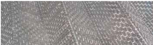
Corrugated textile fabric forming a heat transfer surface area for flat tube air-cooled condensers.
