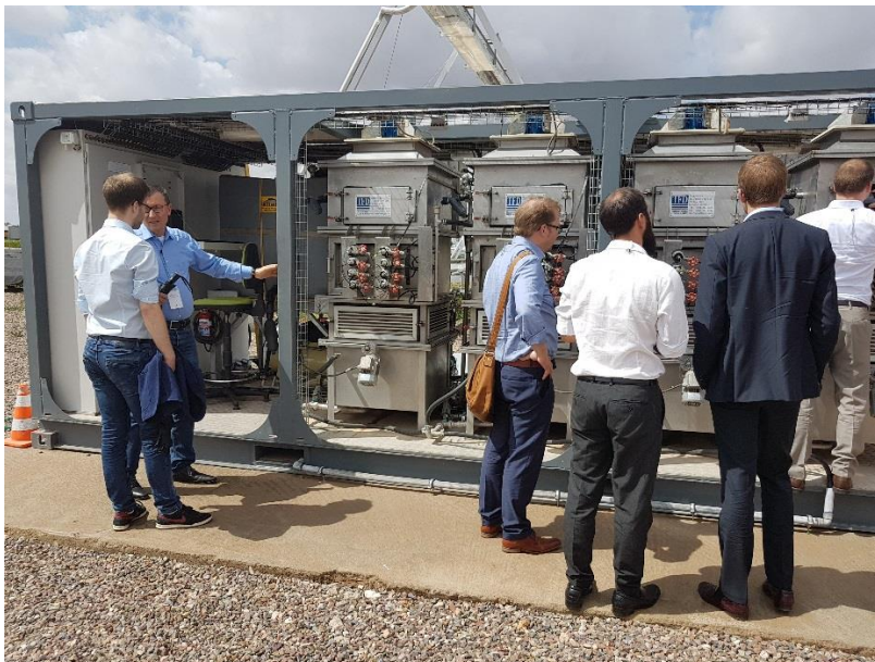
Picture: containerised fouling test rig, consisting of four small deluge cooling towers © Steinbeis 2i GmbH
