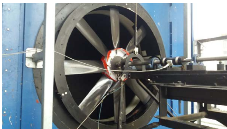
Figure 3: Installed scale fan.
