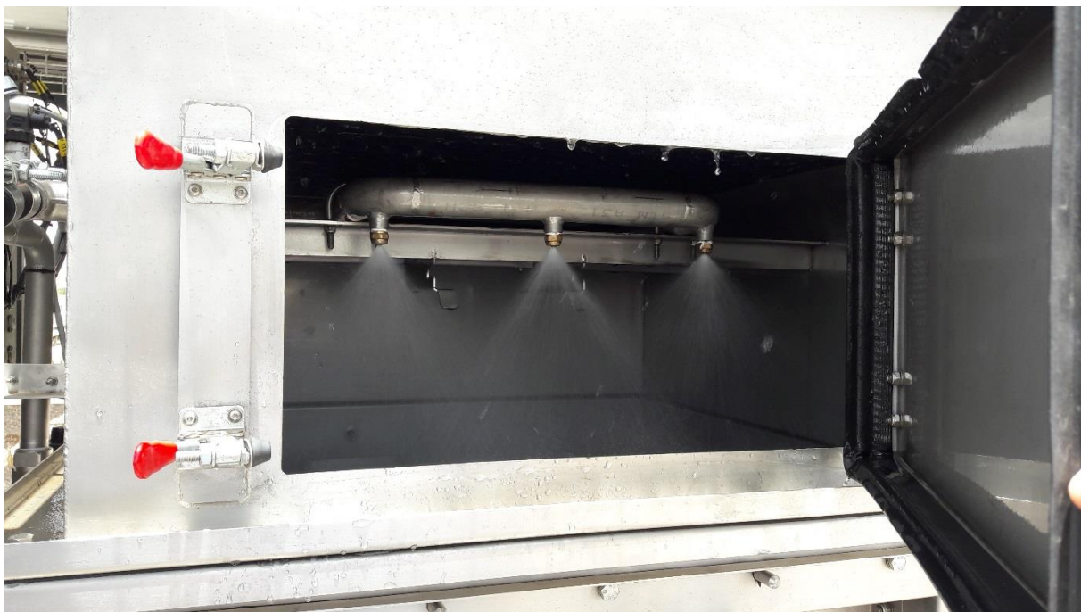
Figure 2.4: Sprayer operation viewed through the top hatch
